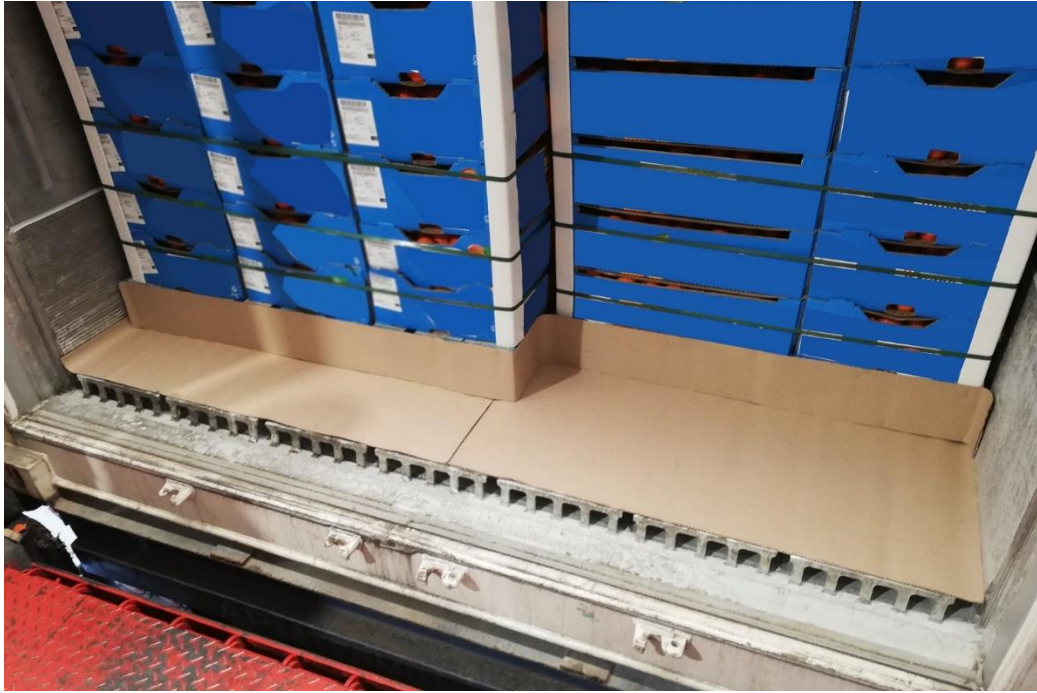
Figure 1: Example of correction installation of void plug.
